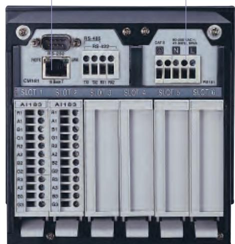
6 SLOTS for Plug & play I/O cards, maximum 6 analog input or mixed with analog & digital I/O cards
